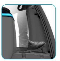
Adjustable pedals The pedals are easily positioned to meet the driver's exact requirements.
